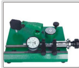
inspect accuracy of dial indicators (range 0-25mm)
