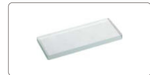
50mm reading scale (check magnification accuracy)
