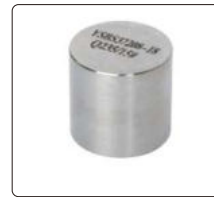
15# carbon steel control sample (optional)
