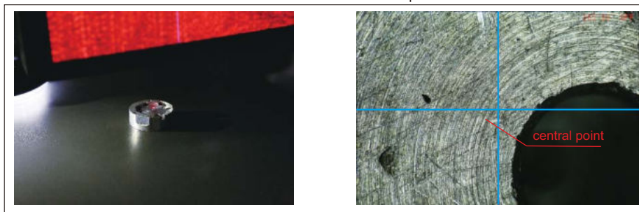
laser indicator locates the central point
