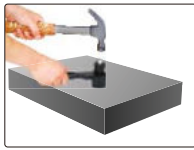
hammer impact to apply test force
